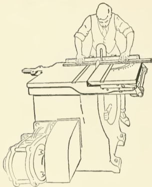
Fig. 37. Cutting with special fence
