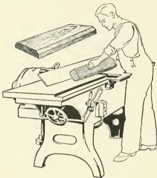
Fig. 41. Cutting bevels on jointer
