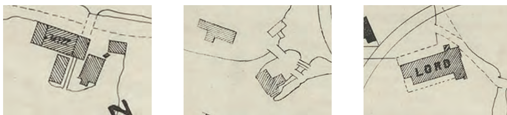
Fig. 2.2.3 1856 plan prepared during planning for the proposed construction of the waterworks showing Lord's lower dams (shaded blue to assist interpretation). The woollen cloth factory ((1) and left detail) was sited at the northern end of the Mill Pond and the flour mill was at the exit to the pond where it emptied into Botany Bay ((2), centre detail). The opening had been dammed by Lord to create the pond system. The location and footprint of Banks House, the Lord's family home, is shown at ((3), right detail). Some of his cottages for workers are also indicated (4), plus Darvall and Castella's large tannery (5). This tannery was situated between today's Byrne and Chegwyn Streets. The northern and southern halves of the Botany area had finally been linked by a bridge over the main pond and the alignment of today's Botany Road identified passing to the tannery.
