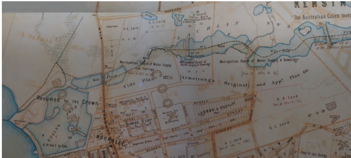
Fig 3.4.3 Most earthworks in the early phase of Botany's development were excavation, not reclamation. Simeon Lord diverted and manipulated the flow of the water in the lower Botany Wetlands to form a series of ponds to use in his mill and factory. These ponds were then enlarged and used by the Waterworks pumping station. (BCHA)
