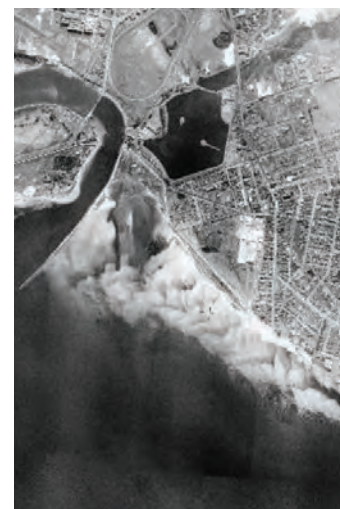
Figure 3.4.6 The 1943 aerial photograph shows how the construction of the sea-wall near Booralee to divert the flow of the Cooks River resulted in major siltation of the bay adjacent to the village with subsequent destruction of the local fishing industry. (NSW LPI SIX maps)
